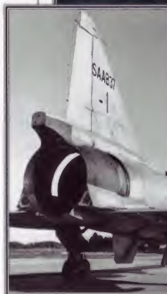
◀ Short landing run Slots in the rear fuselage are connected to the nosewheel and open upon landing to direct the engine thrust forwards.
